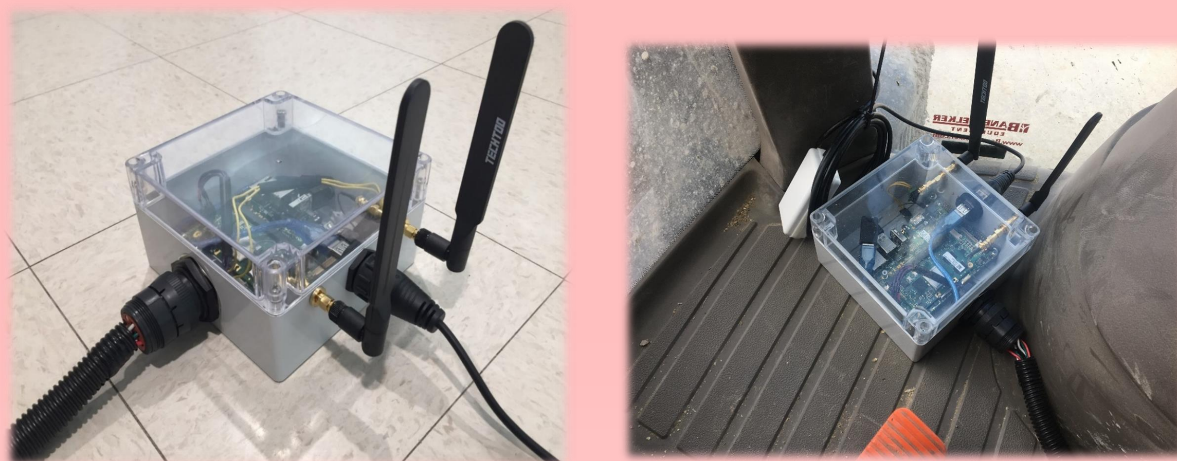
Figure 1 (left to right): an assembled and a deployed ISOBlue 2.0. ISOBlue 2.0 [1] is an open-source ag IoT. It is made to:
