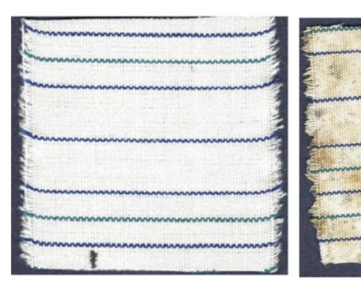
Shirley Soil Burial Test Fabric, used traditionally to measure microbial activity, before and after burial. Threads on the cloth mark areas with standard thread counts, e.g. 36 threads across 1 cm of cloth bounded by two blue threads. This ensures that an equal number of threads are broken in a tensometer during measurement of tensile strength across different soil treatments.
